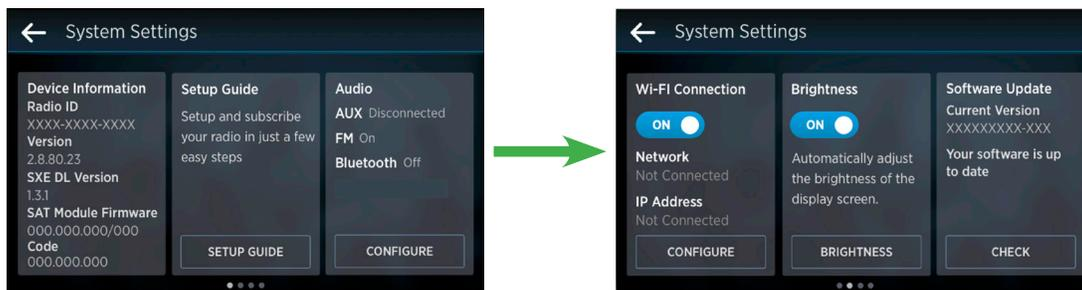
4. Tap the **CONFIGURE** button at the bottom of the Wi-Fi Connection panel.
